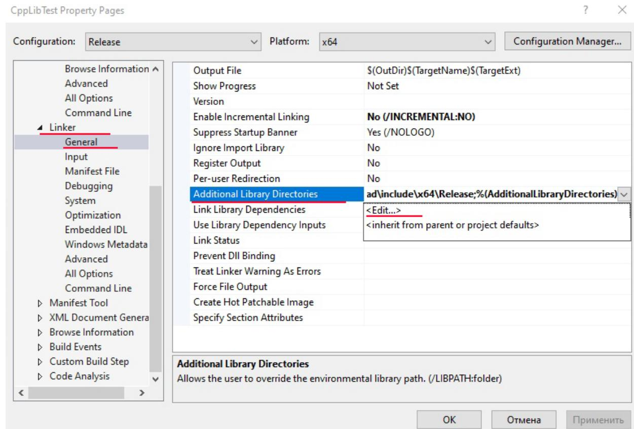
6. Create new line and paste here path to **.lib** file (./robocadSim/Lib/cpp/x64/Release) -> click OK
